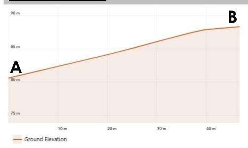
The figure alongside shows the approximate elevation of the site as if it were cut along the above line. It therefor approximates the highest and lowest points along with the slope between them.
